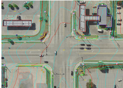
A high-resolution color aerial orthophoto of Sheridan, Wyo., shows planimetric details and contours.
